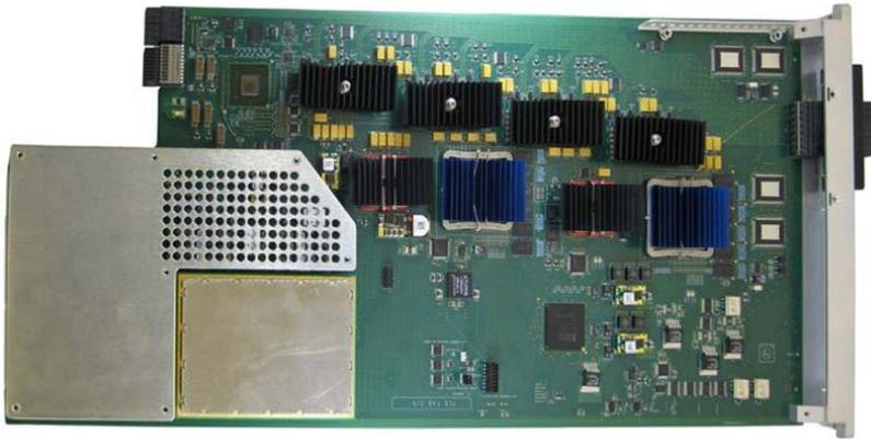
The HSIO is an 8 lane SerDes instrument that is optimized for testing clock-embedded serial interfaces commonly found in modern mobile, consumer, industrial and automotive electronics. These ports connect modems, cameras, displays, and storage to the applications processors to enable high bandwidth, low power consumption, and low EMI.
